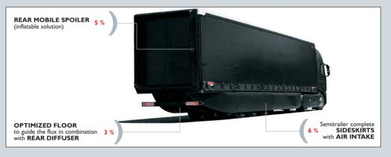
The results of the analysis, realised into Transport Concept, show significant improvements to the power loss due to aerodynamic drag, results that manifest themselves into energy and hence fuel consumption savings.
